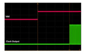
Figure 17. Startup Waveform vs. Vdd
