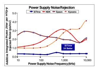
Figure 4. Power Supply Noise Rejection<sup>[4]</sup>
