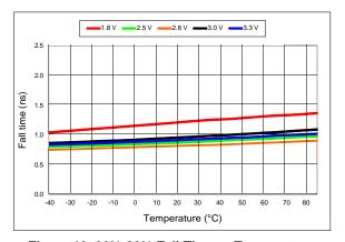
Figure 13. 20%-80% Fall Time vs Temperature
