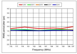
Figure 10. RMS Period Jitter vs Frequency
