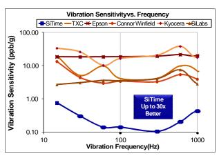
Figure 5. Vibration Robustness<sup>[5]</sup>
