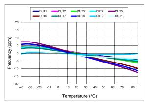
Figure 9. Frequency vs Temperature, 1.8V
