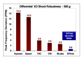
Figure 6. Shock Robustness<sup>[6]</sup>
