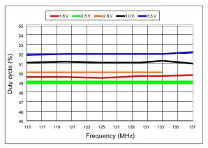
Figure 11. Duty Cycle vs Frequency
