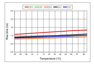
Figure 12. 20%-80% Rise Time vs Temperature
