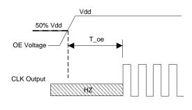
T\_oe: Time to re-enable the clock output
