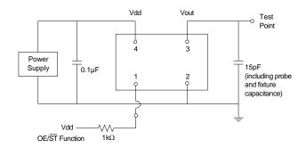
Figure 2. Test Circuit
